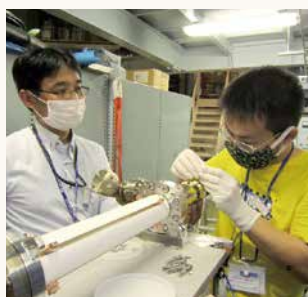
Assembling work of fast beam kicker
