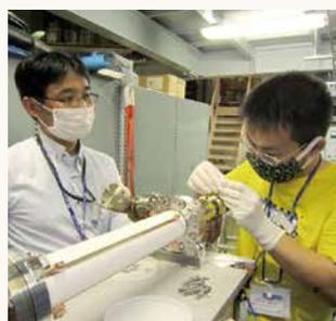
Assembling work of fast beam kicker
