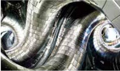
Large Helical Device(LHD)Vacuum Vessel
