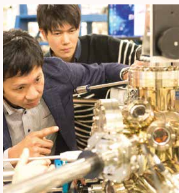
Measurement of the electronic state by photoelectron spectroscopy
