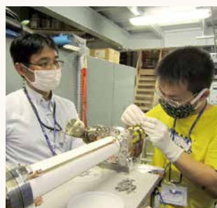
Assembling work of fast beam kicker
